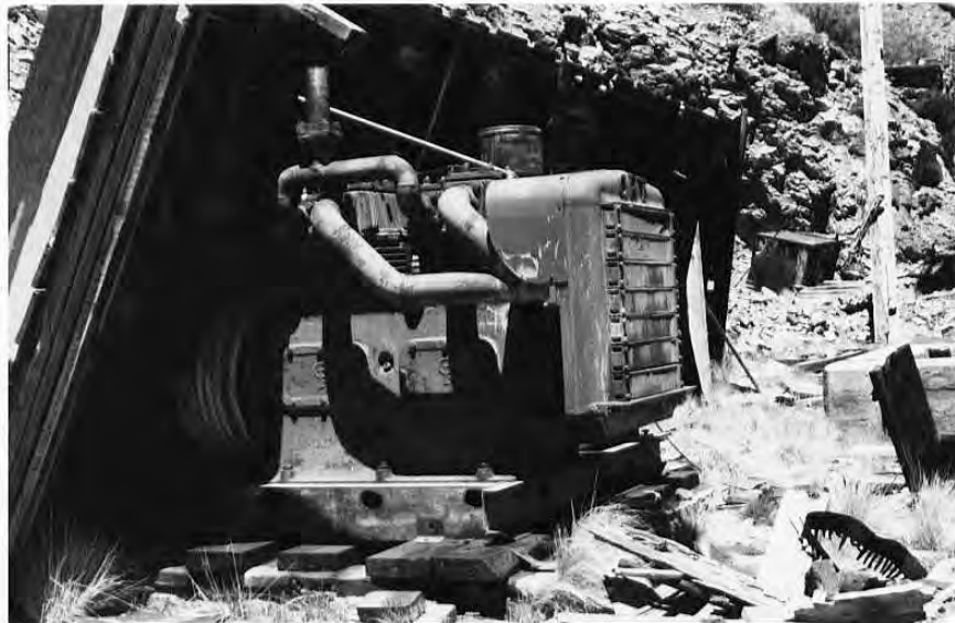
Illustration A 1.4.38: The V-cylinder compressor, similar to a large engine, became one of the most popular compressor types during the 1930s. Note the foundation. Source: Eric Twitty, 1999.
