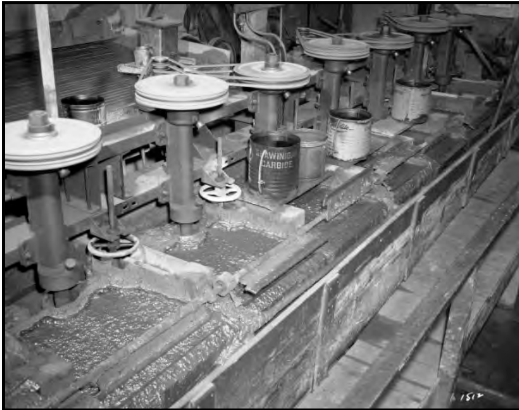
Illustration A 1.4.60: The Alma Lincoln Mill near Idaho Springs was equipped with a battery of flotation cells. Highly efficient, the apparatuses replaced other types of concentration machinery by the 1930s, when the mill was built. The cells were filled with slurry and agitated to a froth. Courtesy of Denver Public Library, CHS.X5495.
