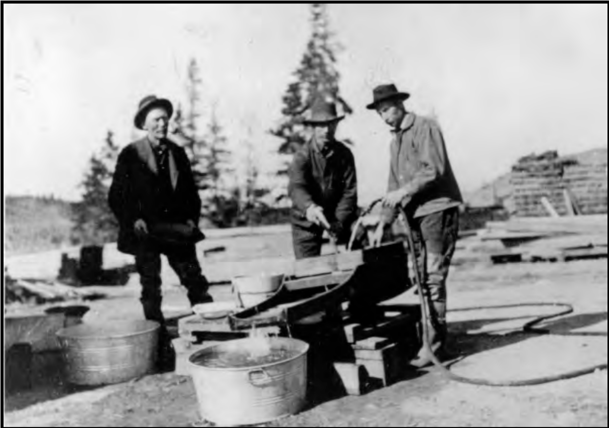
Illustration A 1.4.1: Placer miners near Breckenridge process gravel in a cradle during the 1880s. They shoveled gravel into the hopper at top, flushing it down the riffles with water while rocking the apparatus. The motion caused heavy gold to settle along riffles while light gravel washed through and into the tub. Courtesy of Denver Public Library, X-61131.
