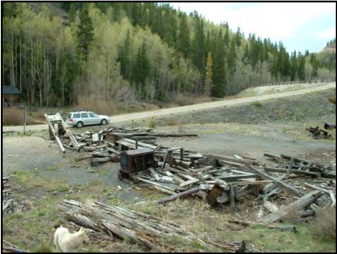
Illustration B 2.3: Sawmill sites today are represented primarily by archaeological features such as foundations, debris, and ruins. The sawmill site in the 2005 photo, near Breckenridge, includes engineered structures and machinery, as well. The object near center is a drive engine, which is rare at sites today. The debris alignment represents a partially intact saw-frame. Source: Eric Twitty.
