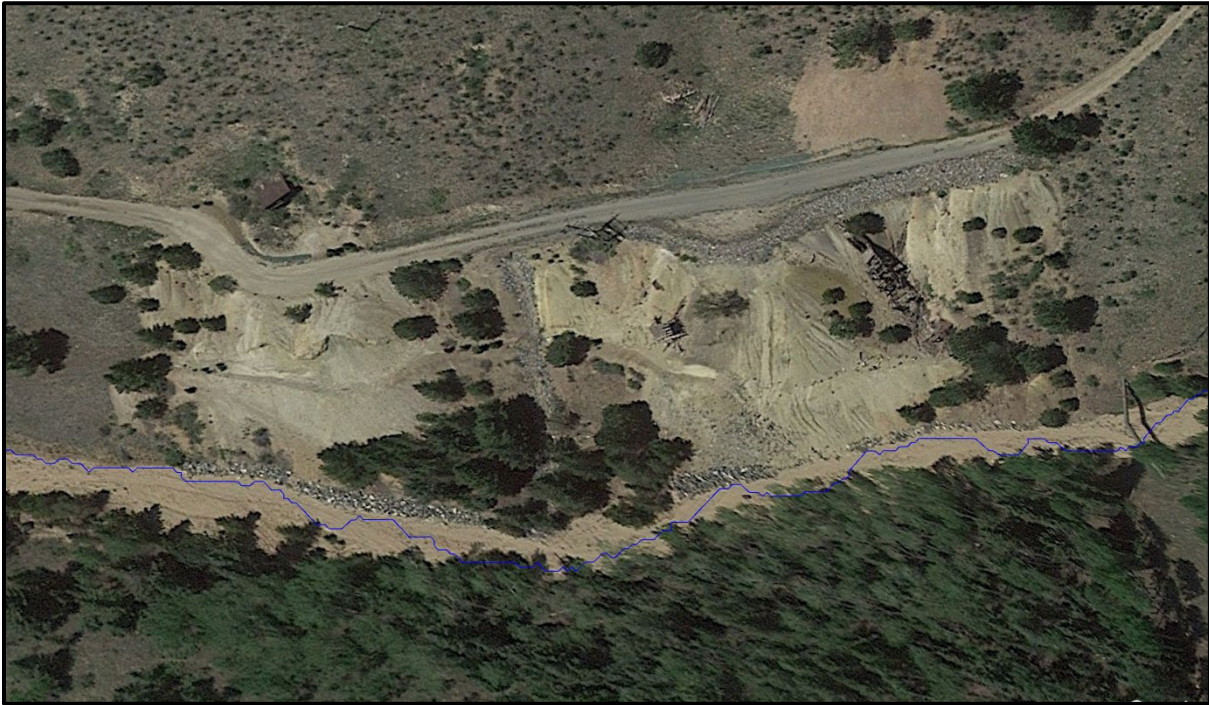
Figure 19. Satellite imagery of the Site #230 waste pile (with numerous rills and gullies visible at the eastern portion) adjacent to Willis Gulch, ~ 700 feet upstream of the confluence with Russell Gulch.
