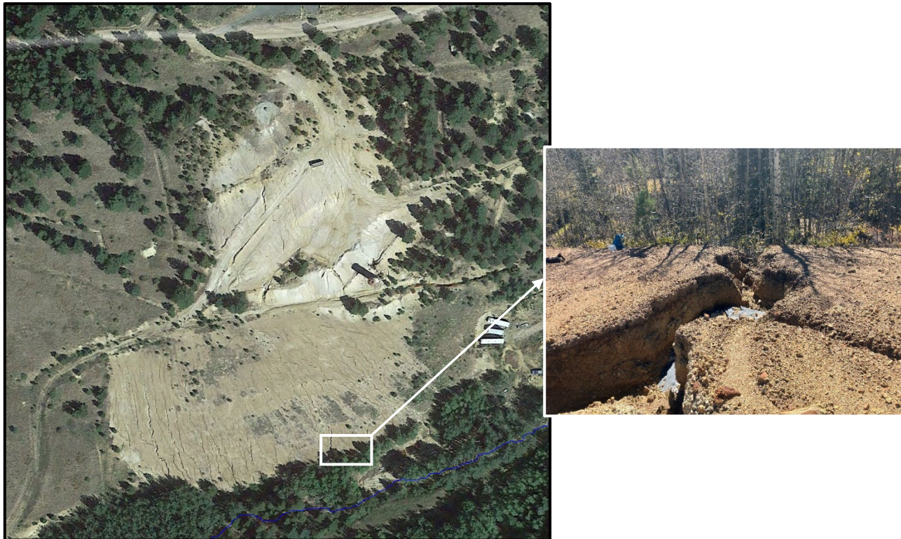
Figure 8. Site #136 - Satellite imagery of the waste pile (with numerous rills and gullies) adjacent to Willis Gulch (left) and significant gully formation along the toe of the waste pile (right).
