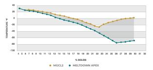
MeltDown Apex gets the job done. The diagram above demonstrates the source of the improved performance of MeltDown Apex. The highlighted gray area is an illustration of the difference in freeze points between MeltDown Apex and MgCl2 when compared at equivalent concentrations.
