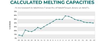
The chart above is an illustraton of the increased melting capacity of MeltDown Apex vs  $MgCl_2$  at a wide range of temperatures. It is this increase in melting capacity that translates to increased efficiencies in deicing operations.
