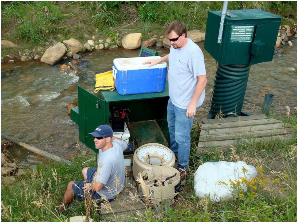
Collecting ambient autosampler samples from CC50
