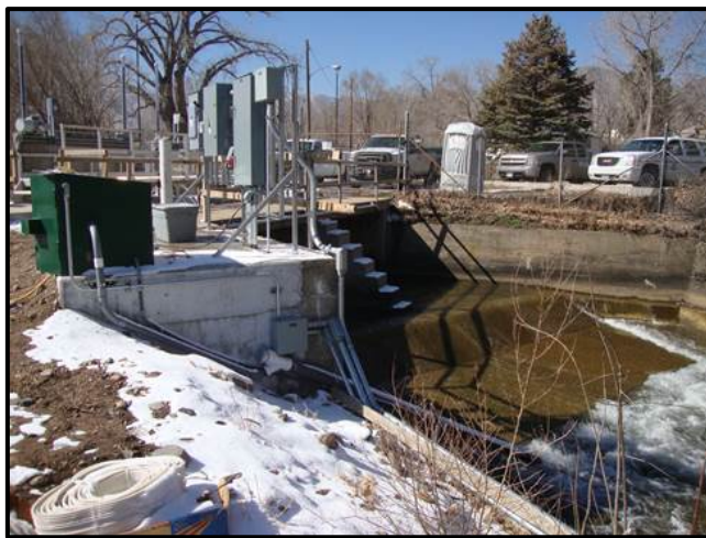
Green Autosampler Box at the reconstructed Farmers Highline Canal headgate. (Photo Credit: Chip Billerbeck)
