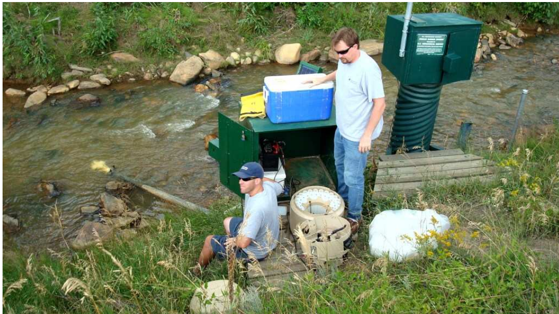
Figure ES-2. Autosampler station on North Fork of Clear Creek (CC AS 50). Gage is the green box on the right, the autosampler is in the middle and the continuous probes/sample collection line is the pipe leading from the creek on the left.
